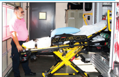
EMT Gary Moore demonstrates how the electric stretchers are raised and lowered hydraulically. All three ambulances include this feature now.
